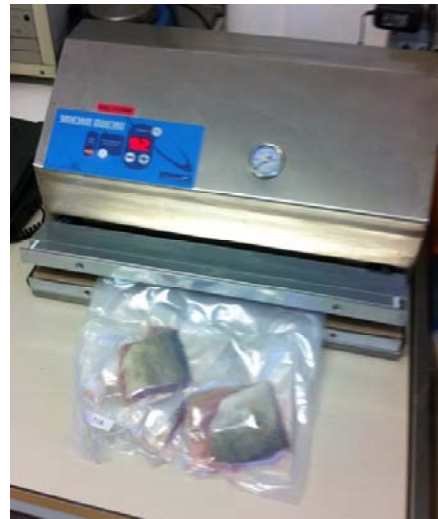
Figure 4. Fish fillets sandwiches are packed under vacuum
